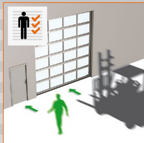
Completely separate doors for pedestrians and goods.
