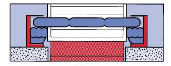
Furthermore, the cushions cannot get into the lorry opening like it is common with the curtain-type dock shelters. Consequently, an optimal accessibility of the lorry bed as well as a maximum operating range on the ramp can be guaranteed. For dock shelters up to an outer height of 4700 mm integrated inflatable rear bottom cushions are standard resulting in optimum sealing of the whole system. Power supply system: Protection IP 65, 230/400 V - 50 Hz.
