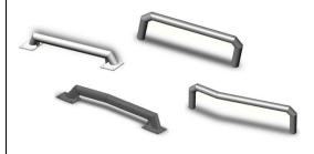
Wheel guides help the truck driver to reverse to the loading bay without any complicated maneuvering actions. They are installed on yard level, either by being cast directly into concrete (types PEK and PEKE) or by being bolted on the ground (types PEF and PEFE); they represent a good and reasonable investment into the safety at your loading bay.
