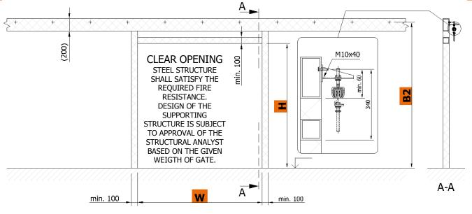
Construction readiness of the opening is secured by the customer according to the requirements of the contractor and depending on the type of jamb and lintel of the opening.
