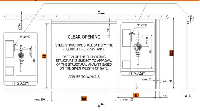
Construction readiness of the opening is secured by the customer according to the requirements of the contractor and depending on the type of jamb and lintel of the opening.
