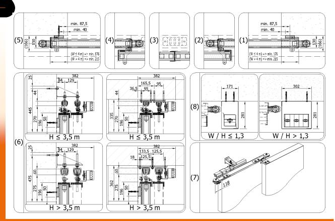
Minimum required dimensions of steel structure
