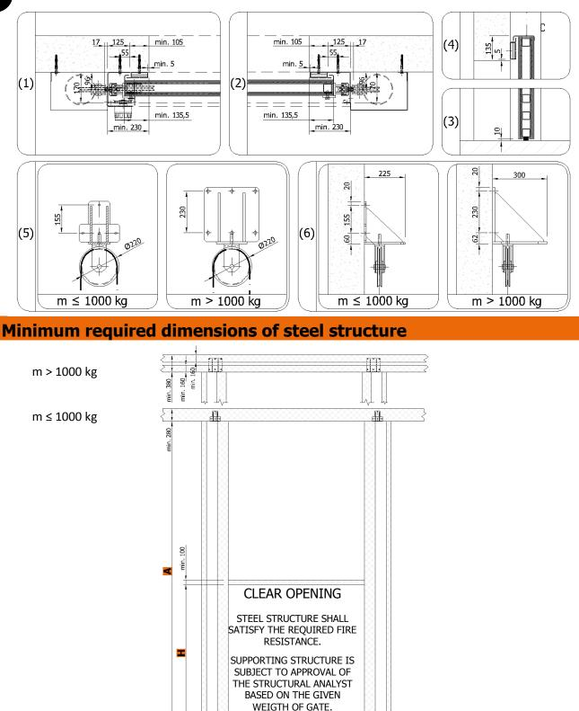
Construction readiness of the opening is secured by the customer according to the requirements of the contractor and depending on the type of jamb and lintel of the opening.
