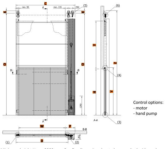
Minimum height  $H_{min}$  = 2000 mm. Smaller dimensions has to be consulted with producer.
