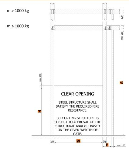
Construction readiness of the opening is secured by the customer according to the requirements of the contractor and depending on the type of jamb and lintel of the opening.
